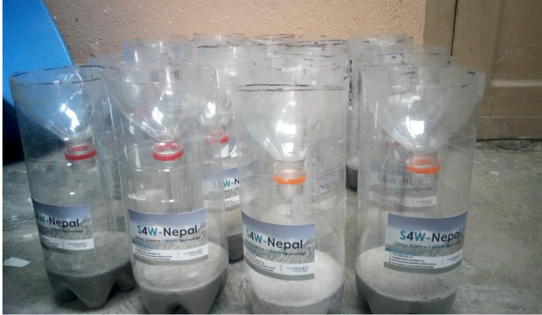
Figure 1: Cheap Soda Bottle Rain Gauges Made by S4W-Nepal for Measuring Precipitation
