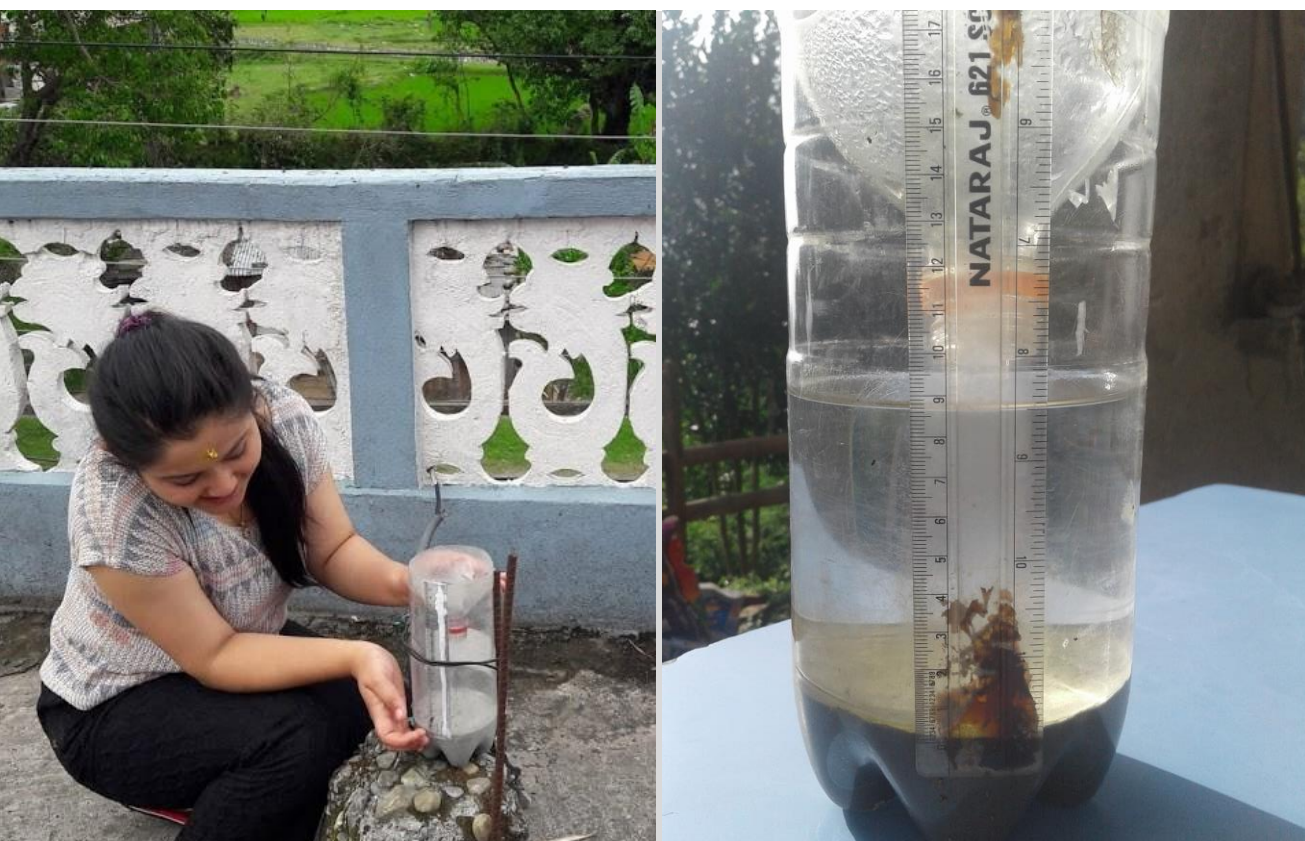
Figure 2. S4W-Nepal CS and recycled rain gauge.
