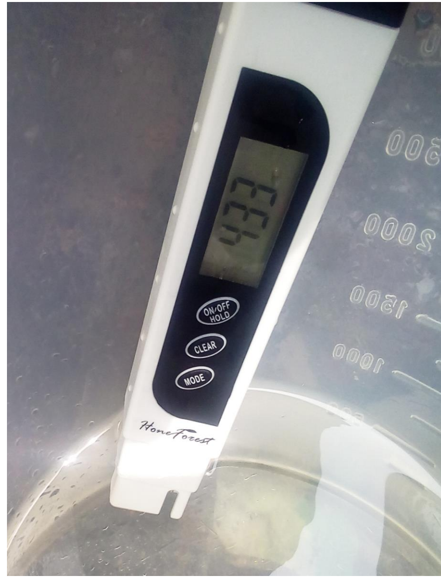
Figure 3. Measurement of stone spout discharge and EC.
